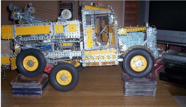
to my wife's annoyance! The back axle unit has probably been rebuilt eight times at least, as the model became increasingly heavier. Scammell's walking-beam concept is very clever but puts great strain on the half-shafts, which are now heavy-duty items on the model. At the front, the axle is not just driven but steered too, of course, and a typically
